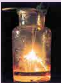
图3-3-3 铁丝在氧气中燃烧
