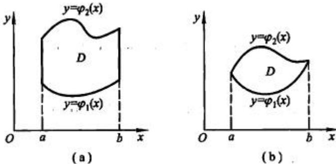
$$\iint_D f(x, y) dx dy = \int_a^b dx \int_{\varphi_1(x)}^{\varphi_2(x)} f(x, y) dy \quad (\text{先固定 } x, \text{ 得到 } y \text{ 范围再确定 } x \text{ 可移动范围})$$
